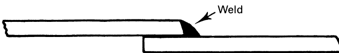
FIGURE 5-11 An old method of tank construction allows liquid to enter the gap between the plates.
