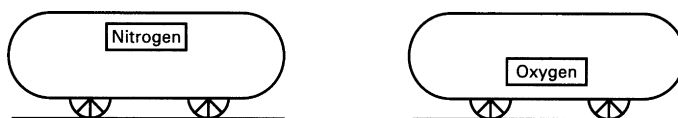
FIGURE 4-2 Arrangement of labels on tank cars. The Nitrogen label folds down to read Oxygen.
