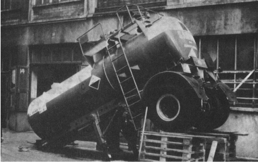
FIGURE 13-1 A tank trailer may tip up if the rear compartments are emptied first.
