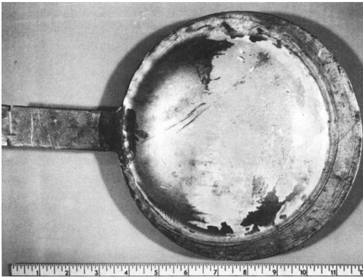
FIGURE 1-6 A slip-plate bowed by a gauge pressure of 470 psi (32 bar).
