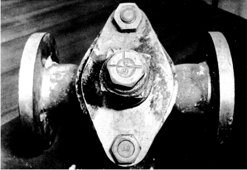
FIGURE 25-3 The central bolt was marked to show the position of the cock. When two washers were inserted under the bolt, it could not be screwed down as far as before and the marks no longer corresponded with the position of the cock.
